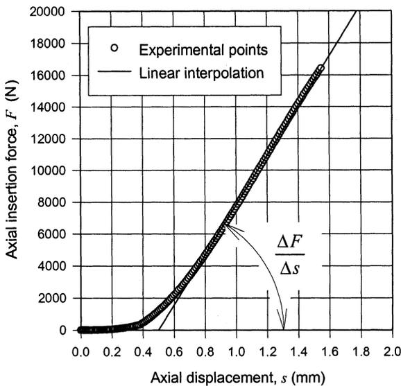
**FIGURE 3** Typical plot of insertion force against axial displacement at assembly of a taper press fit.
