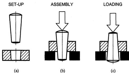
**FIGURE 2** Geometry of specimens with assembly and loading arrangements.
