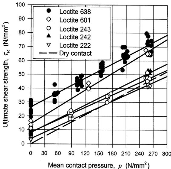
**FIGURE 1** Variation of ultimate shear strength with contact pressure for dry and bonded annular butt joints.
