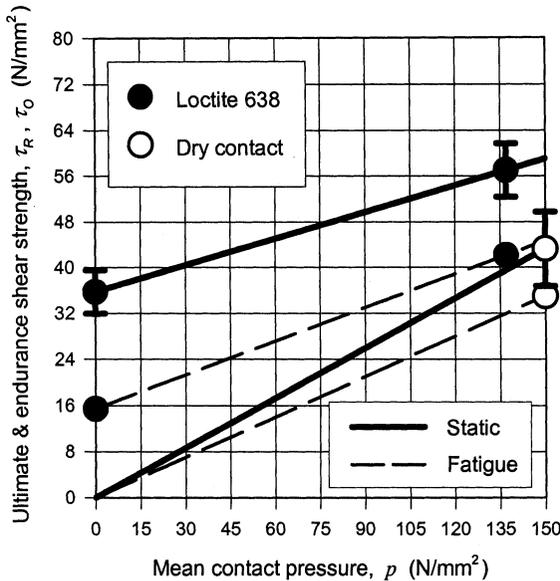
**FIGURE 6** Comparison between static and fatigue strength for dry and bonded taper fits.
