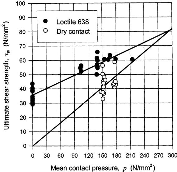
**FIGURE 5** Variation of ultimate shear strength with contact pressure (from Equation (A3)) for dry and bonded taper fits.
