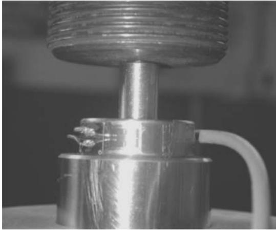
**FIGURE 4** Closeup of a collar instrumented with an electrical-resistance strain gauge.
